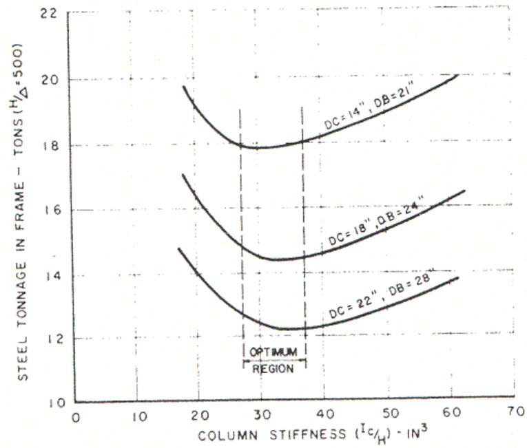
Figure 4 - Optimum beam and column stiffness
