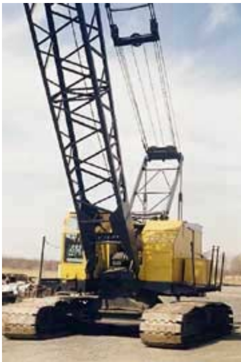
Lattice Crawler Crane
