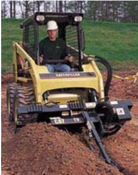
Skid Steer with Trencher
