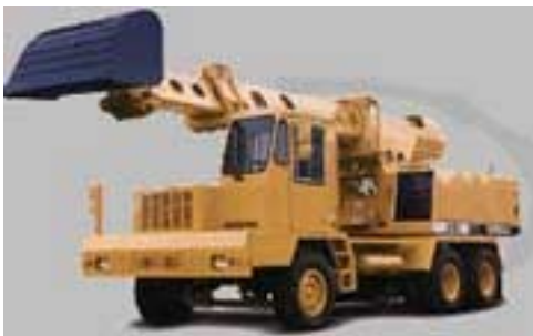
Gradall Truck Trencher
